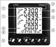
3. Unit (V, A, PF, Hz, kW, kVAr, kVA) Indicates unit of parameter displayed
