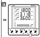
Press P (←) button, the eighth screen shows: [ Max Active, Reactive, Apparent demand Power (kW, kVAr, kVA)
