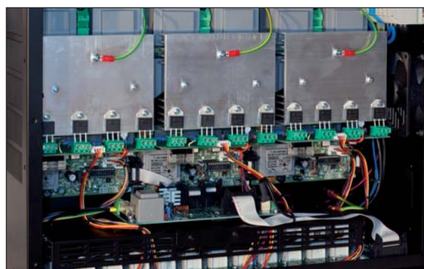
Inside view. Pegasus dimmers are modular with easily replaceable parts.
